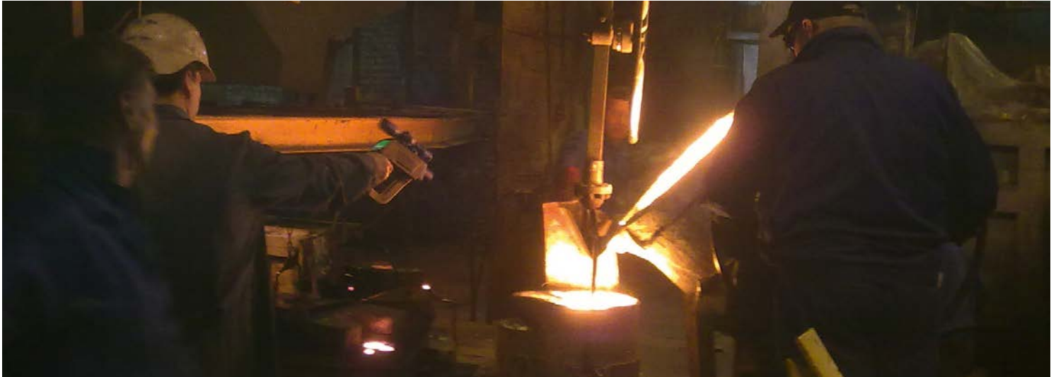
Detailed infrared temperature measurement on a melt in the casting plant with P20 05M.
